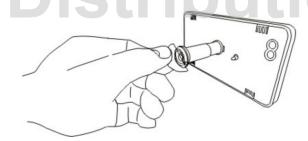
• Insert the batteries on main unit and place onto the back cover
