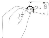
• Use the tool provided in the kit to tighten the lens
