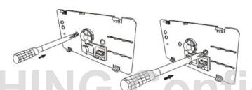
Insert tube and turn counter clockwise
